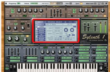
The LCD screen in the middle of the user interface contains seven master sound effects and an arpeggiator. The master effects are applied at the end of the audio path. Each effect has its own settings panel on the LCD screen. To switch between the different effect panels, click on the name of the effect on the left side of the screen.
