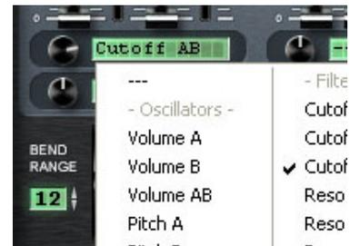
You can set the amount of modulation for each parameter using the small rotary knobs next to the destination displays. Turning them to the right results in a positive modulation value, turning them to the left gives a negative value. The middle position is the default position and means there is no modulation. If you double-click the knob it will jump back to this default position.
