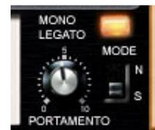
There are two portamento modes, *Normal (N)* and *Slide (S)*, which can be selected using the *Mode* switch right next to the portamento knob. In *Slide* mode it will always slide the pitch to the next note played. In *Normal* mode however, it will only slide notes whenever at least one other key is pressed, but it will not slide when you play a single note at a time.
