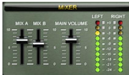
On the right side of the Mixer panel is a VU meter which measures the output level. Please note that it is in general not a problem when the red LEDs are lighting because the output of Sylenth1 is not clipped. The host software can turn the volume down if needed to prevent clipping.
