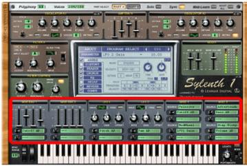
The modulation panel enables you to modulate a whole set of parameters using two ADSR envelope generators, two Low Frequency Oscillators and a set of other sources. Each source can be linked to two different parameters, which can be chosen from a popup menu that appears when you click on one of the destination displays.
