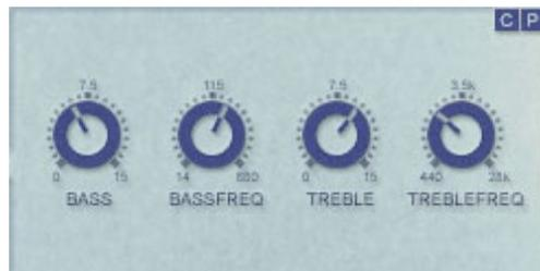
If the *Bass* and *Treble* knob are both set to 0, the sound will be unchanged. Note that the equalizer will automatically normalize the volume level whenever bass or treble is added.
