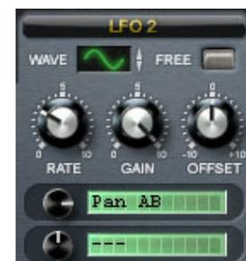
0. If the Free button is pressed, the LFO will run freely and will not be retriggered when a new note is played, nor will it sync to the host tempo.
