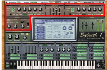
As said before, there are two *Part* sections on the Sylenth1, named *A* (red) and *B* (yellow), which can be switched using the part select buttons. Each of these parts contains two oscillators, a filter panel and an amplitude envelope.
