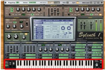
The keyboard section at the bottom of the user interface consists of a 5-octave keyboard, a pitch bender, a modulation wheel and portamento controls.
